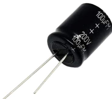
Polar fixed capacitors are intended for indoor installation with resistance requirements to high humidity of 98% at the temperature 35°C, for operation in direct and pulse current circuits of radio electronic equipment. Sealed. In insulated case with radial wire leads.
